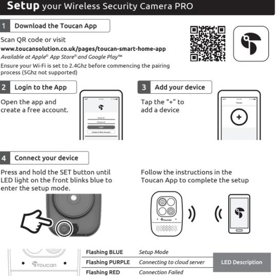
LED Description: Flashing BLUE Setup Mode, Flashing PURPLE Connecting to cloud server, Flashing RED Connection Failed
