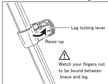
To adjust leg extension, raise up Leg Locking lever and extend legs to the desired position then lock. Use upper part legs when it is not necessary to extend all legs till the maximum height.
