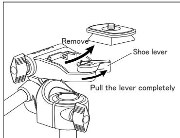
Raise up Shoe Lever until lock is released. Slide out the Quick-release to remove.
