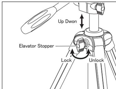
Unlock elevator stopper, and rotate Crank handle to up or down to the desired height. Then lock the Elevator stopper.
