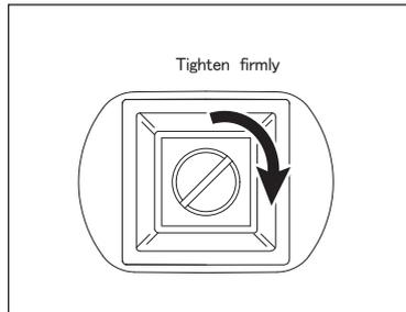
Adjust the screw to the bottom of camera body, then tighten with screw driver firmly.
