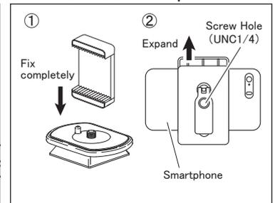
In case of taking picture with smartphone, fix enclosed smartphone holder with camera screw firmly. Then extend smartphone holder like above arrow's direction and set firmly. \*Screw hole locate at bottom and back side of smartphone holder, so please use depended on situation.
