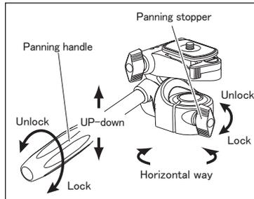
Unlock the Panning handle by twisting to anti-clockwise direction, and can move Up-and down. Unlock Panning stopper, and can move to horizontal.
