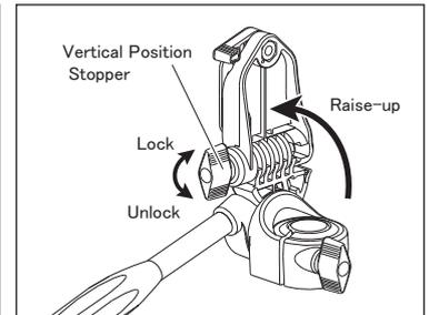
Unlock the Vertical Position stopper, and turn camera plate to vertical position to 90° degrees for the portrait photo.
