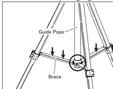
When opening the leg, brace stopper should be end of guide pipe. If it isn't that, push brace down, then reach to end of guide pipe. (Finally brace stopper make more steady.)
