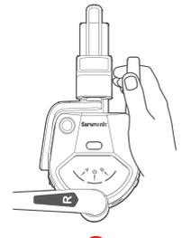
4. While using, please do not cover the antenna area shown in the figure above to avoid signal interference, and do not handle the antenna to avoid damage.
