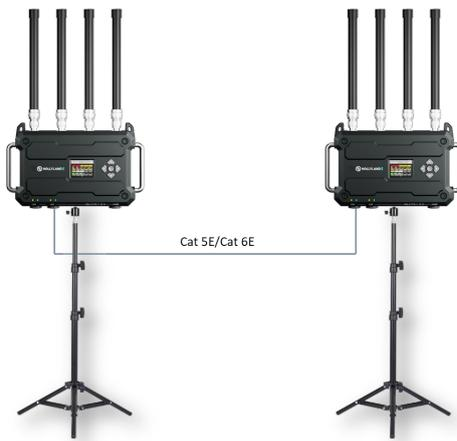
It does only support 2 hubs connection. On one hub, select **Master Device**, and on another hub, select **Remote Device**.
