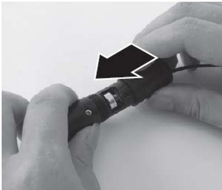
3. Place the new battery, with the + and - oriented as indicated, into the battery compartment in the power pack. The + symbol is stamped outside the compartment for reference.
