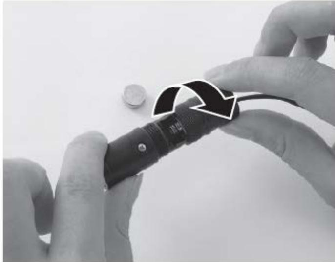
2. Remove the old battery from its compartment in the power pack.
