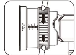
When adjusting the spot light, to adjust the beam angle of light, turn the dial on the lens with two fingers, like adjusting zoom on a camera lens to get the focusing effect. (As described on the light.)
