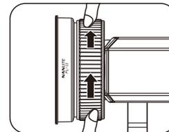
When adjusting the flood light, to adjust the beam angle of light, turn the dial on the lens with two fingers, like adjusting zoom on a camera lens to get the flooding effect. (As described on the light.)
