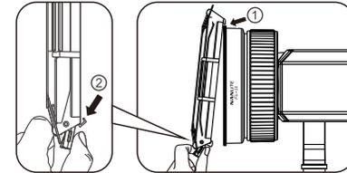
When installing the barn door, make sure the mount points ① of barn door connect properly in place onto this rim of the fresnel, pinch the mount points ② of barn door with hand and clamp it onto the Fresnel Lens. (As described on the light.)
