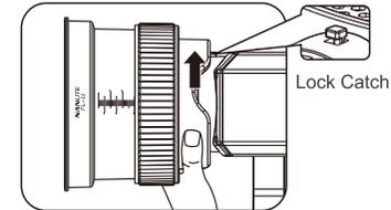
When removing the fresnel lens, push and hold on the lock catch while rotating the lens and you are able to remove it from fixture.
